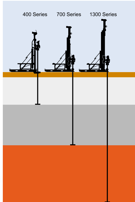
The LM's deep hole capacity is shown graphically above. The chart shows the relative depth capacity for the Boart Longyear LM family of diamond drills.
